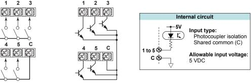
Dielectric strength: 500 VDC for one minute (between input terminals and the ground terminal)
